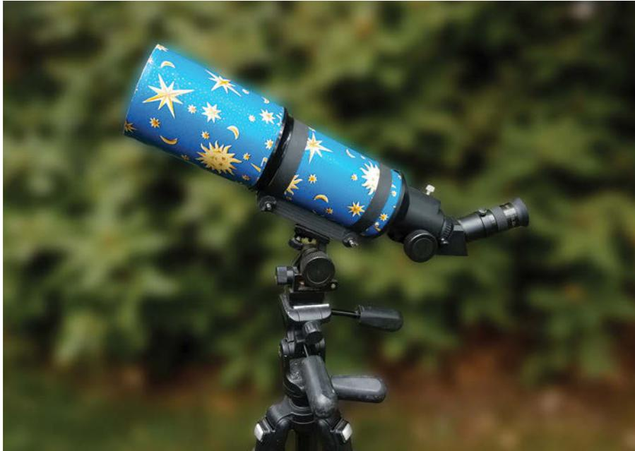
◀ An 80-mm refractor offers a fine — and inexpensive — view of the night sky. Use an erect-image diagonal (shown here), and it makes a great terrestrial scope, too.
