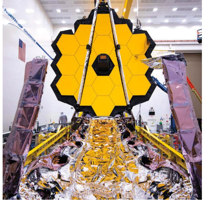
▲ **SEMI-DEPLOYED** The sunshield lies furled below the unfolded primary mirror. For launch, the shield will fold up and sandwich the mirror.
