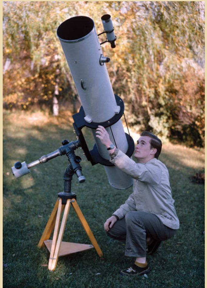
▲ **HOMEBUILT PIPE-MOUNTED “CAVE”** Coauthor Klaus Brasch with the 8-inch f/7 Newtonian he built in using Cave optics. The scope rides on an iron pipe equatorial mount — something commonly described as a “plumber’s nightmare.” He fashioned other components out of wood, sheet metal, and assorted hardware as suggested in the now-classic *Amateur Telescope Making* book series.
